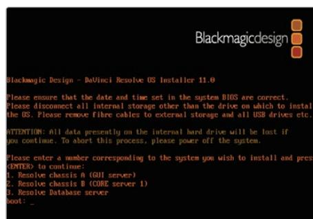
**Step 6.** The installer permits multiple server configurations to be made however we are only interested in #1, the Chassis A GUI server.
