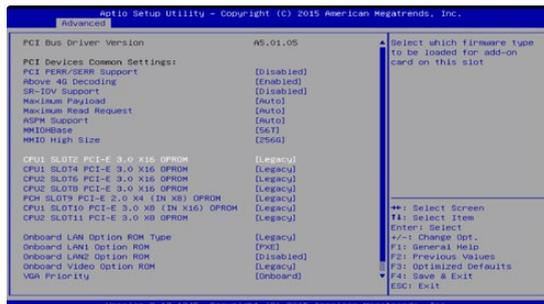
Step 9. With the slot 4 line selected hit 'Enter' and then using the arrows or -/+ keys select disable and then 'Enter' to go back to the list.
