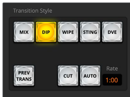
The Auto transition button is part of the Transitions Style group
