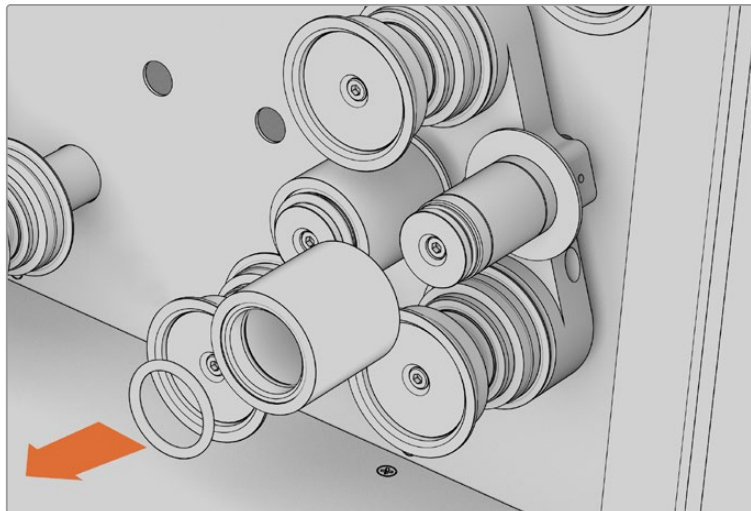
To clean the particle transfer rollers, simply remove the O-ring at the end of each PTR spindle and slide off the roller
