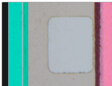
Correct 8mm film edge setup. The overlay is aligned to the edge of the film reference edge. The transparent overlay touches the film ref edge correctly.
