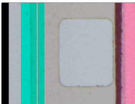
Incorrect 8mm film edge setup. The overlay is not aligned to the edge of the film reference edge.
