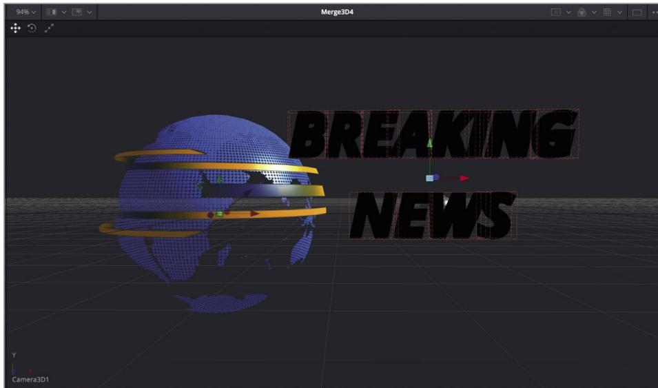
The text appears black in the frame because the lights are not being passed through the merge nodes. Before you continue animating the text, let's enable the lights to pass through to merge 3D 4.
