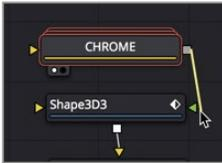
The rectangles now get a reflective chrome material applied. Adding material to 3D text requires a slightly different technique. The 3D text node requires you to put a replace material 3D node after it to apply the material to the text.
