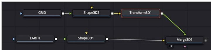
Inserting a transform 3D node adds a second *pivot point* to the grid. The grid has its own pivot point based on the shape 3D node that acts as the grid's axis of rotation. The transform 3D node adds an additional pivot in the center of the 3D world that will act as the grid's orbital center.
