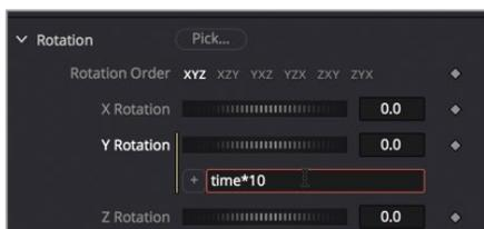
Although this procedure may seem cryptic at first, it is easy to understand. Because this field is for Y rotation, all of its values refer to degrees of rotation. Entering time tells the Y rotation parameter to change its value as the playback advances frame-by-frame. At frame 1 the rotation value will be  $1 \times 10$  degrees, and at frame 10 the rotation value will be  $10 \times 10 = 100$  degrees of rotation around the Y axis.
