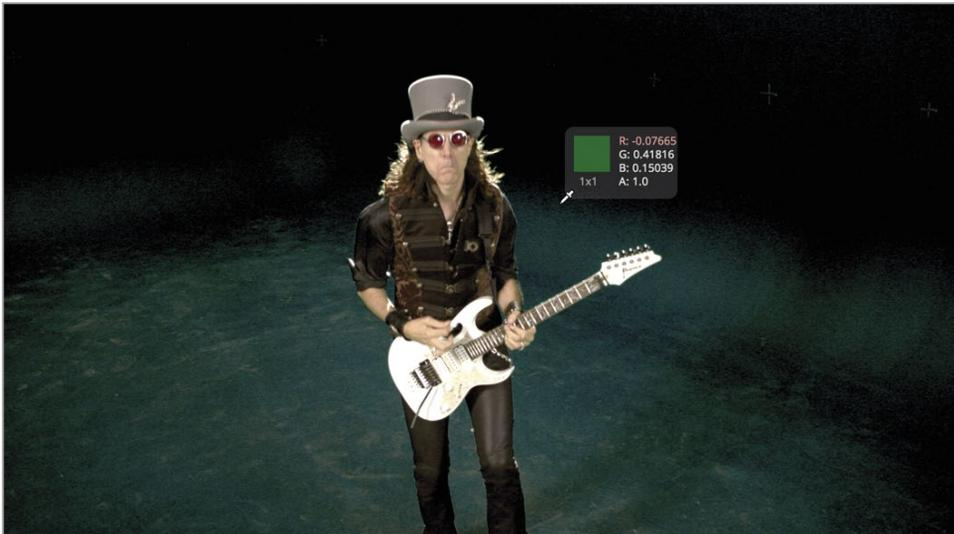
**TIP** When sampling an area of the frame for a key color, select an area where the audience will be focusing its attention in the final shot. Doing so sets you up for creating an optimal key.
