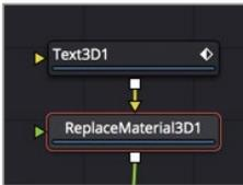
The replace material node has only one connection other than the yellow input where the text is connected. The green replace material input is used as the input for the material you want to use.
