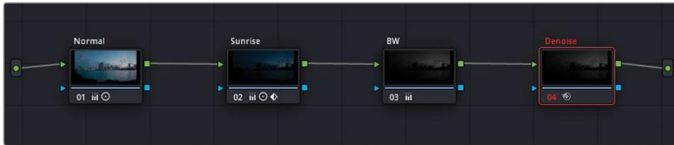
This time, the change prompts the Denoise node to turn red and require a new cache. The BW change affected the RGB input of the Denoise node, which has to perform a new render using the new RGB signal.
