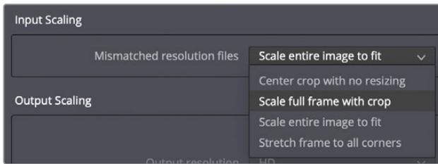
Scaling full frame with crop ensures that the longest dimension of the timeline viewer is filled with the source media, removing letterboxing or pillars. However, this often means that a small portion off the top and bottom of the image will be cropped.
