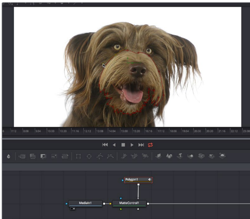
A node tree for doing a simple rotoscoping job
