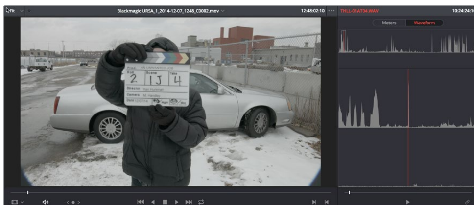
Aligning video and audio sync points with the Audio Panel set to show the Waveform panel
