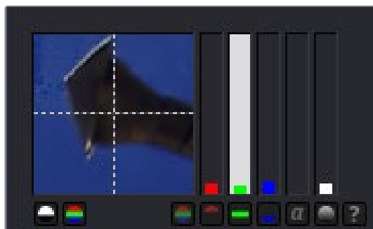
Channel bars indicate which channel is selected for tracking
