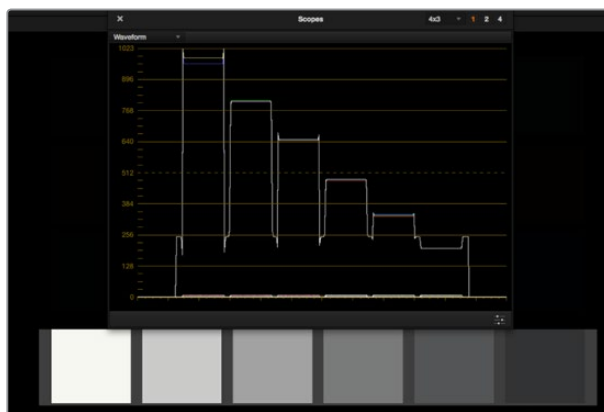
(Left) Poorly lit chart with irregularly topped waveforms, (Right) Well lit chart with flat-topped waveforms
