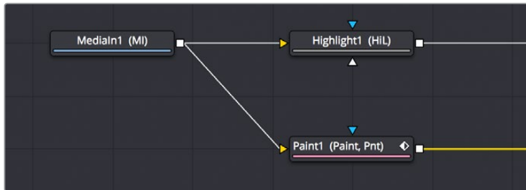
One node branching to two to split the image to two operations
