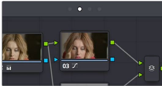
Four dots at the top of the Node Editor let you choose which mode you're working on
