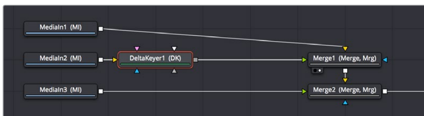
Adding a DeltaKeyer node inline after the MediaIn2 node
