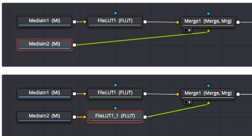
Copying a node from one part of the node tree and pasting to insert it into after a selected node
