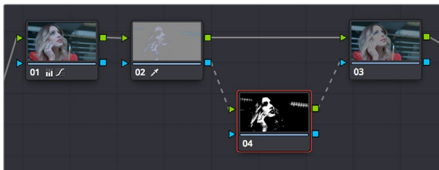
Connecting a key output to an RGB input to adjust a key with a second node's controls
