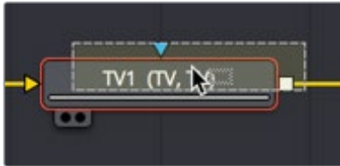
Dragging a node from the Effects Library onto a node in the Node Editor to replace it
