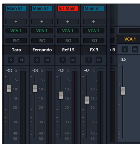
Adjusting the VCA 1 fader also adjusts the Tara, Fernando, Ref LS and FX3 faders that are assigned to that VCA.
