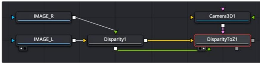
A Disparity to Z node creates an image with a Z channel.
