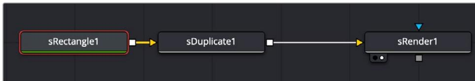
An sRectangle node connecting to an sDuplicate node, and then viewed using an sRender node
