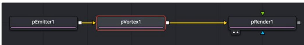
A pVortex node creates a spiraling motion for particles that fall within its pull.
