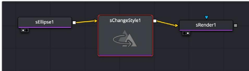
A simple node tree showing the sChangeShape node taking the output of an sEllipse shape, performing the style change, and passing it to the sRender node.
