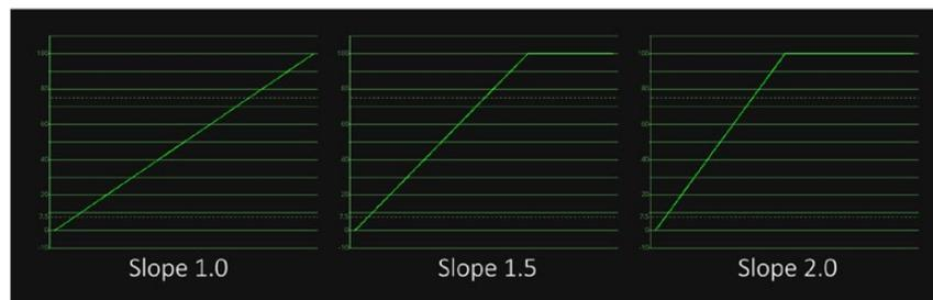
Slope multiplies the color values; this is the same as Gain in the Brightness Contrast node.
