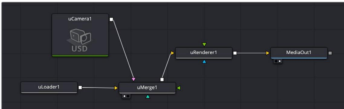
The uCamera node is connected to a uMerge node to give standard camera controls to a USD scene.
