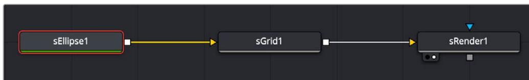
An sEllipse node connecting to an sGrid node, and then viewed using an sRender node
