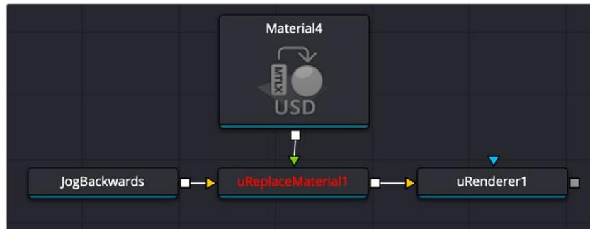
A node tree showing a MaterialX definition (.mtlx) file called Material4 loaded into a uMaterialX node, then passing that material to a uReplaceMaterial node to change the material in a USD scene called JogBackwards.
