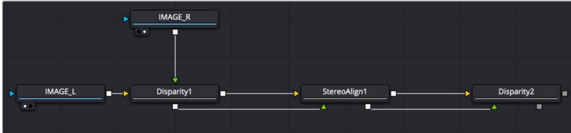
A Stereo Align node destroys the disparity channel, so another Disparity node is placed after it
