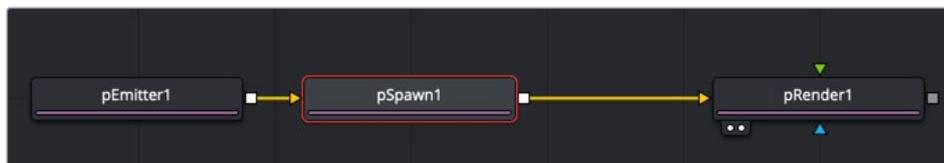
A pSpawn node used to generate new particles at specific points in the old particles' life
