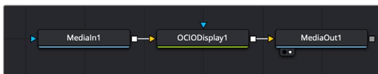
A simple node tree showing the OCIO Display node taking the Media In Node, performing the Display Transform, and passing it to Media Out
