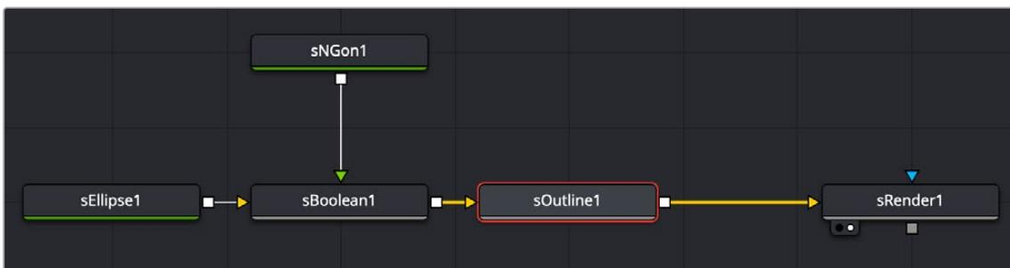
A compound shape from an sBoolean node is connected to an sOutline for creating a complex outlined shape
