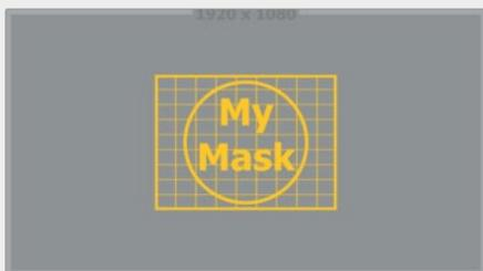
**Stretch:** The image source is stretched in X and Y to accommodate the full dimensions of the generated mask. This might lead to visible distortions of the image source.
