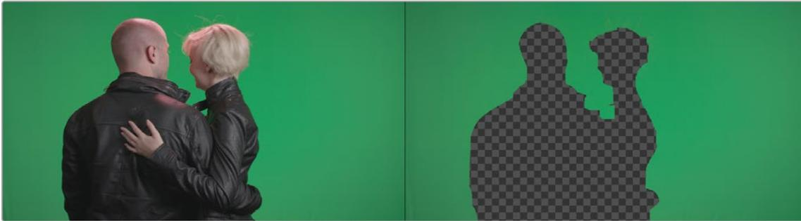
Once you have the selection, the Erode control expands the pre-matte, removing any small pixels of non-green/blue screen around the edges. Then, growing the pre-matte fills in the holes until you have a solid blue or green image.
