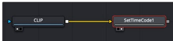
A Set Timecode node inserts new timecode metadata into the background clip.
