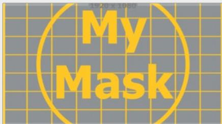
**Height:** The image source is scaled uniformly until its height (Y) fits the height of the mask. Depending on the relative dimensions of the image source and mask, the image source's X dimension might not fit the mask's X dimension, resulting in either cropping of the image source in X or the image source not covering the mask's width entirely.
