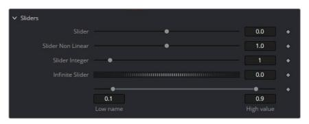
Sliders can be integer or floating point, can also be a fixed range or unlimited range, can be scaled or fixed scale, can have fixed limits and can also operate non linearly.
