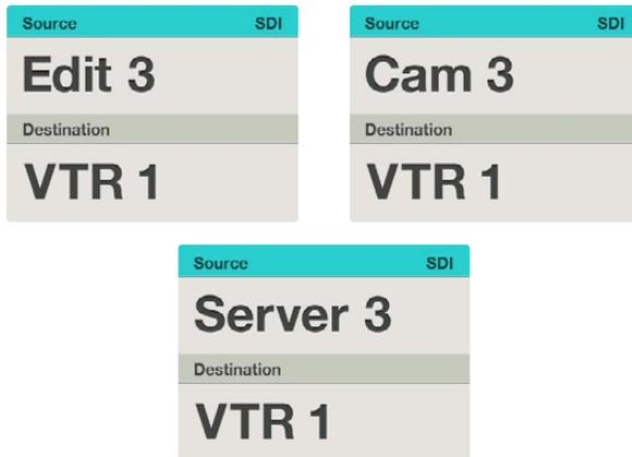
In this example, the numeric button "3" has been selected so only video sources with a "3" in their label will be listed, on the LCD, when the scroll wheel is rotated. This provides a fast way to find a video source because you only have to scroll through a short list of equipment based upon a group number, e.g. only list the equipment in Studio 3.
