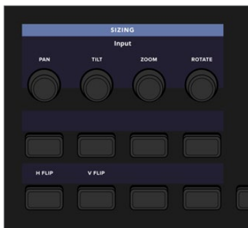
The unlabeled "More" key found to the bottom left of each of the side panel soft menu controls lets you choose an alternate or second set of controls for that panel's current menu.
