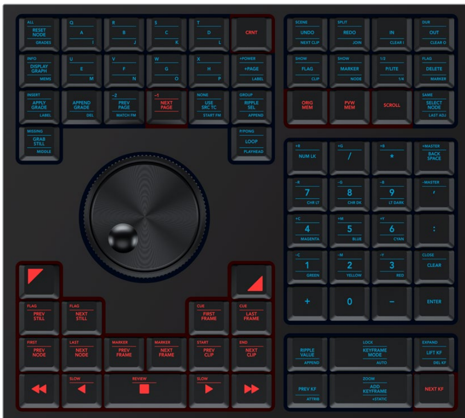
Pressing SHIFT DOWN highlights all keys with alternate SHIFT DOWN functions so you can instantly see which keys are selectable.
