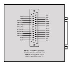
Pinout diagram of the DB25 connector
