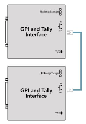
Daisy chain multiple GPI and Tally Interfaces using Ethernet. Power must be supplied to each individual unit in the chain.
