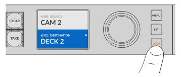
To prevent routes from being switched on a specific output, press the lock button to lock the output
