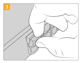
Replace the keycap by aligning it onto the button and gently pushing until you feel it click into place.
