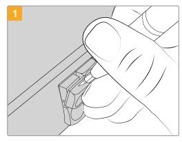
The button keycaps can be easily removed using a small flathead screwdriver.
