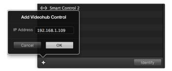
Press the + (add device) button and enter the IP address of a GPI and Tally Device you want to add. Press the Identify button to activate the LED on a selected GPI and Tally Interface.
