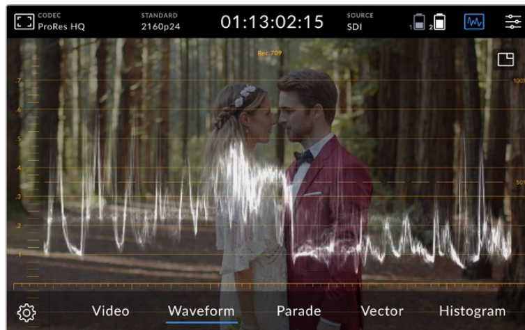
The waveform display showing luminance values
