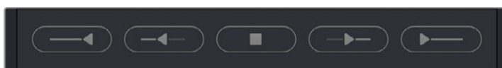
The analysis buttons, left to right: Track from Last Frame, Track Backward, Stop Tracking, Track Forward, Track from First Frame
