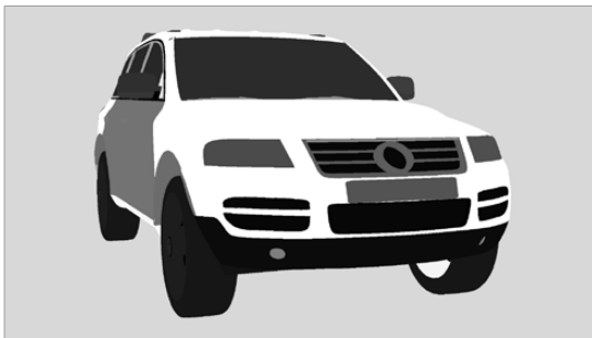
Object ID for ground plane and object set to the same numeric value
