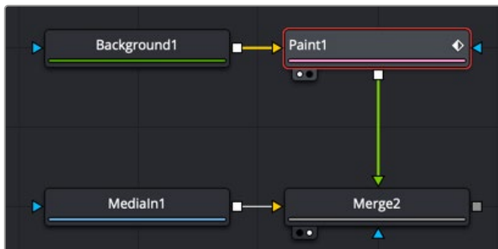
A Paint node merged over the top of a MediaIn for more flexibility
