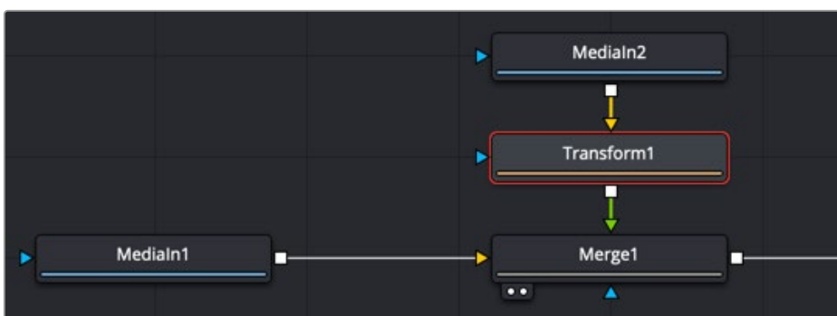
The Transform node can be used to scale an image without changing its resolution.
