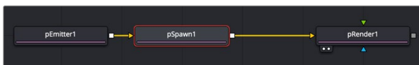
A pSpawn node used to generate new particles at specific points in the old particles' life
