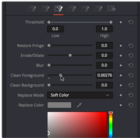
Adjusting the Clean Foreground slider in the Matte panel of the DeltaKeyer controls
