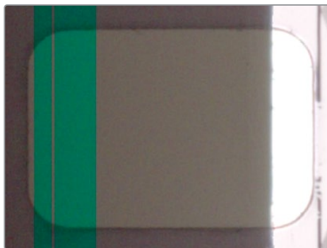
Incorrect 16mm setup. The overlay is not aligned to the edge of the perforation. With the 16mm HDR skid plate installed, the stabilizer aligns automatically to the other side of the perforation to avoid interfering with the film image and improve horizontal stability. When using a 'non-HDR' 16mm skid plate, it functions the same as the 35mm skid plate.
