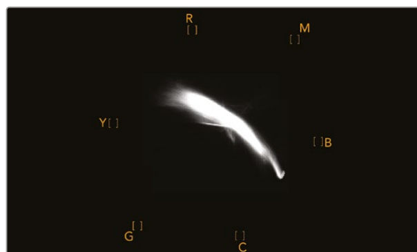
Vectorscope display showing the "fleshtone line" towards the 10 o'clock position
