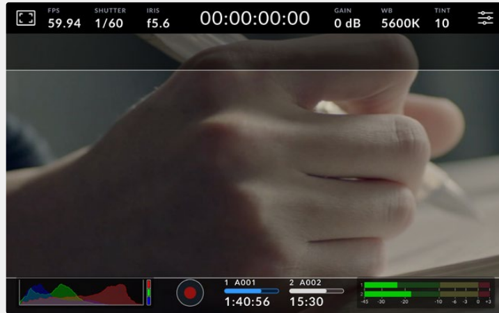
The LCD touchscreen with 2.40:1 frame guides enabled
