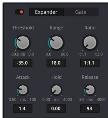
Fairlight Expander/Gate parameters in the Dynamics window
