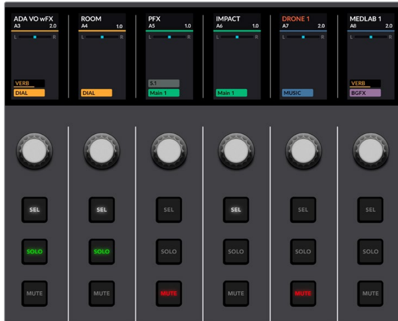
Desktop Console with active Mute, Solo, and Select buttons in the fader channel strips
