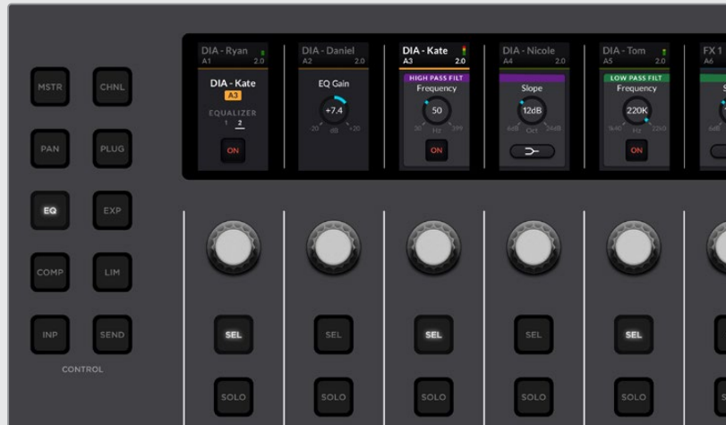
EQ control set Page 2 with controls for the filters on Bands 1 and 6
