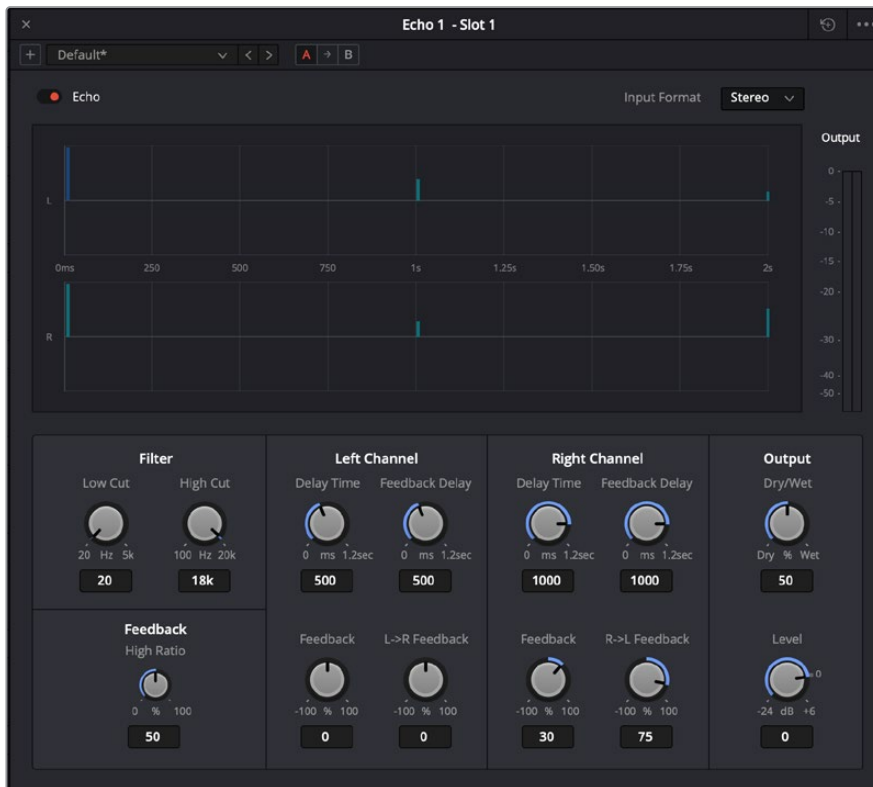
Echo Plugin window that mirrors the Plugin control set on the Fairlight Desktop Console
