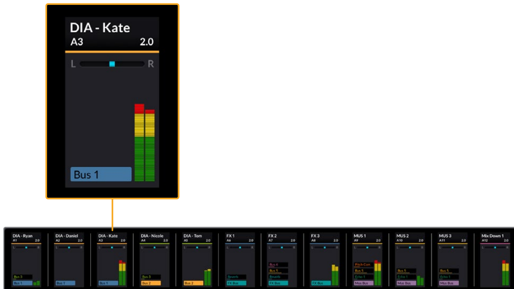
Fader channel strip LCD screens showing track name, number, channel format, color, pan status, bus assignments, and level meters.
