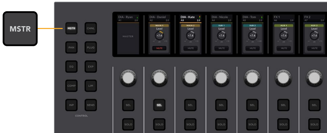
Master control set mapping shows MAIN 1, MAIN 2, SUB 1, SUB 2, AUX 1, and AUX 2
