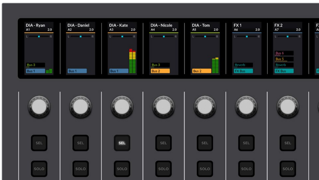
Control buttons that assign control sets to the adjacent Select buttons, knobs, and LCDs
