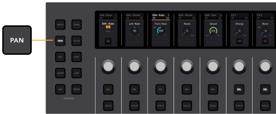
Pan control set mapping includes all parameters in the Fairlight Pan window.
