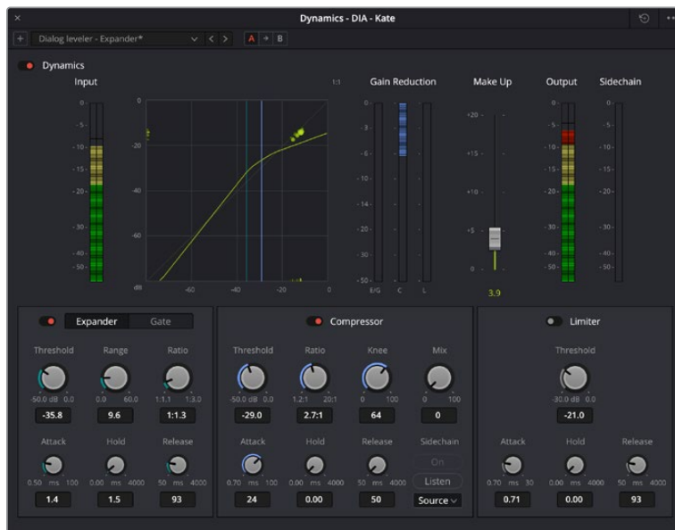
Fairlight Dynamics Window, which includes Expander, Gate, Compressor, and Limiter.
