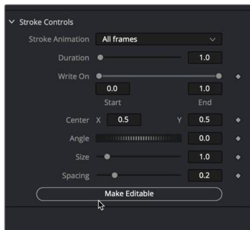
The Stroke's control points can be revealed using the Make Editable button
