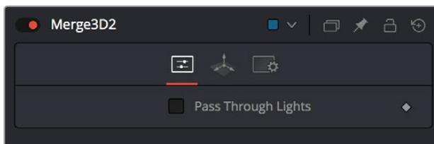
You can light downstream Merge3D scenes with lights connected to upstream Merge3D scenes by turning on Pass Through Lights
