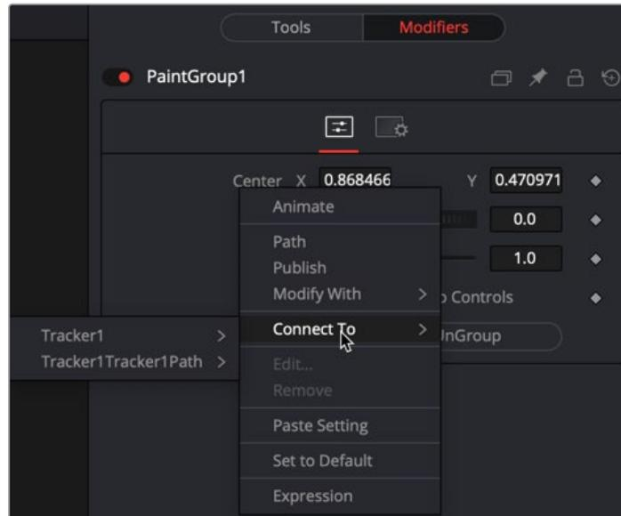
Use the onscreen controls, or in the Modifiers tab, right-click over the Paint Group's Center X label to connect the tracker
