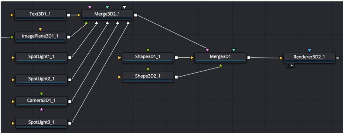
You can build elaborate scenes using multiple Merge3D nodes connected together
