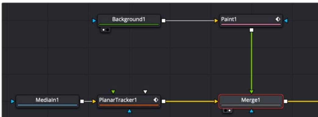
Paint node merged over the top of a steadied Planar Tracker
