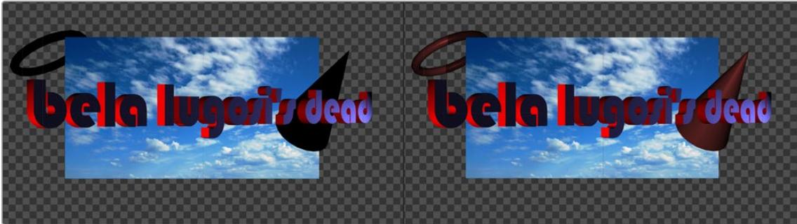
The result of lights on the text in one Merge3D node not affecting the cone and taurus added in a downstream Merge3D node (left) Turning on Pass Through Lights in the upstream Merge3D node results in those lights also illuminating the downstream shapes (right)
