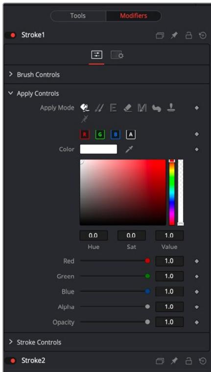
Once you stop painting a stroke, it's added to the Modifiers tab along with an additional Stroke modifier that represents the next stroke. For instance, if you paint your first stroke, the Modifiers tab shows your stroke as Stroke1 and then a stroke 2 as well, which represents the next stroke you create. You always have one more stroke in the Modifiers tab than strokes in the viewer.
