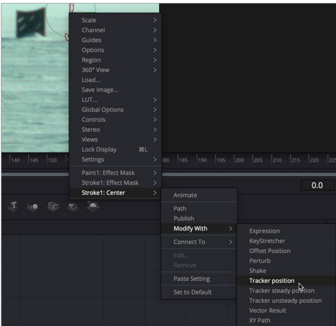
Right-clicking over the Stroke's Center control in the view allows you to apply a tracker modifier
