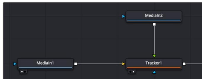
Tracker node connected serially so it can both track and transform the input images
