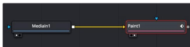
The Paint node is inserted directly after the node it is painting on
