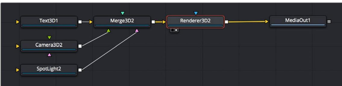
Output of a Merge3D connected to a Renderer3D node to output 2D image data
