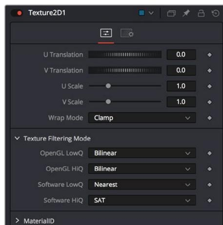
The Texture2D node is used to translate a texture in the UV space of the object, as well as set the filtering and wrap mode
