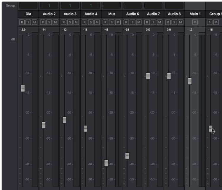
Adjusting the Group 1 fader also adjusts the faders for Audio 1, 3, and 4 that are assigned to that group
