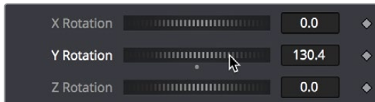
Thumbwheel controls for X,Y and Z rotation with arrows on either end for fine tune adjustments
