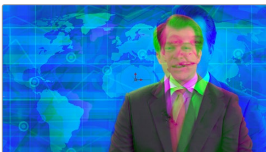
Transforming only the green color channel of the image with a Transform effect
