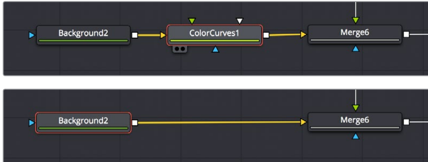
(Top) Before deleting a node from a node tree, (Bottom) After, upstream and downstream nodes have automatically reconnected
