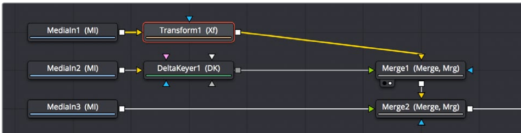
Adding a Transform node to change the sizing of the Medialn1 image connected to the background
