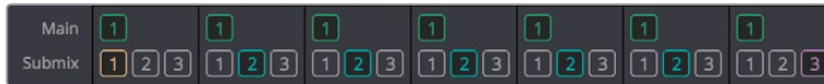
Main and Submix buttons let you assign tracks to buses, and buses to other buses
