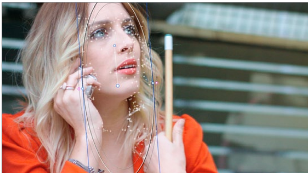
Object tracking in progress. Tracking points are automatically placed over trackable features of the image
