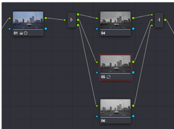
Adding the Splitter/Combiner nodes to use Node Sizing on individual color channels
