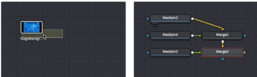
(Left) Dragging three nodes from the Media Pool to the Node Editor, (Right) Merge nodes are automatically created to connect them all
