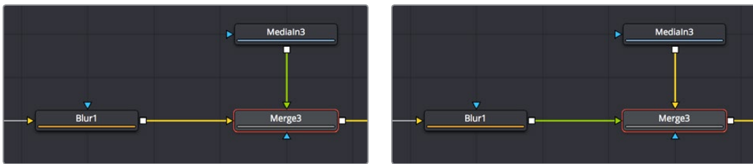
(Left) Before swapping node inputs, (Right) After swapping node inputs, connections don't move but the colors change
