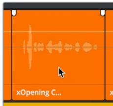
Fader handles appear when you hover the pointer over a clip
