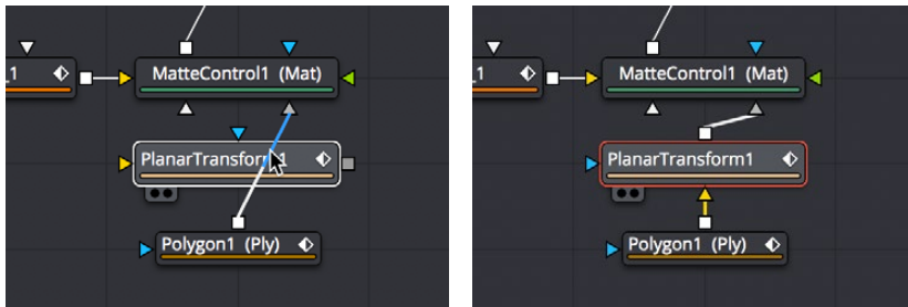
(Left) Inserting a PlanarTransform node by holding the Shift key down while dropping over a connection, (Right) After inserting the PlanarTransform mode
