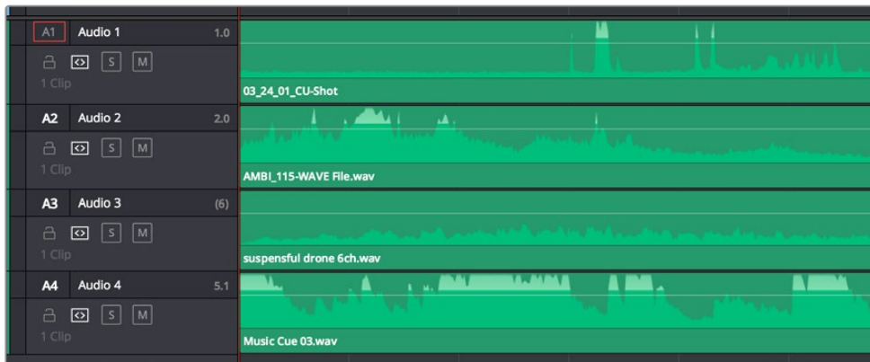
Four audio tracks with a variety of audio tracks shown. From the top down, Mono, Stereo, Adaptive, 5.1
