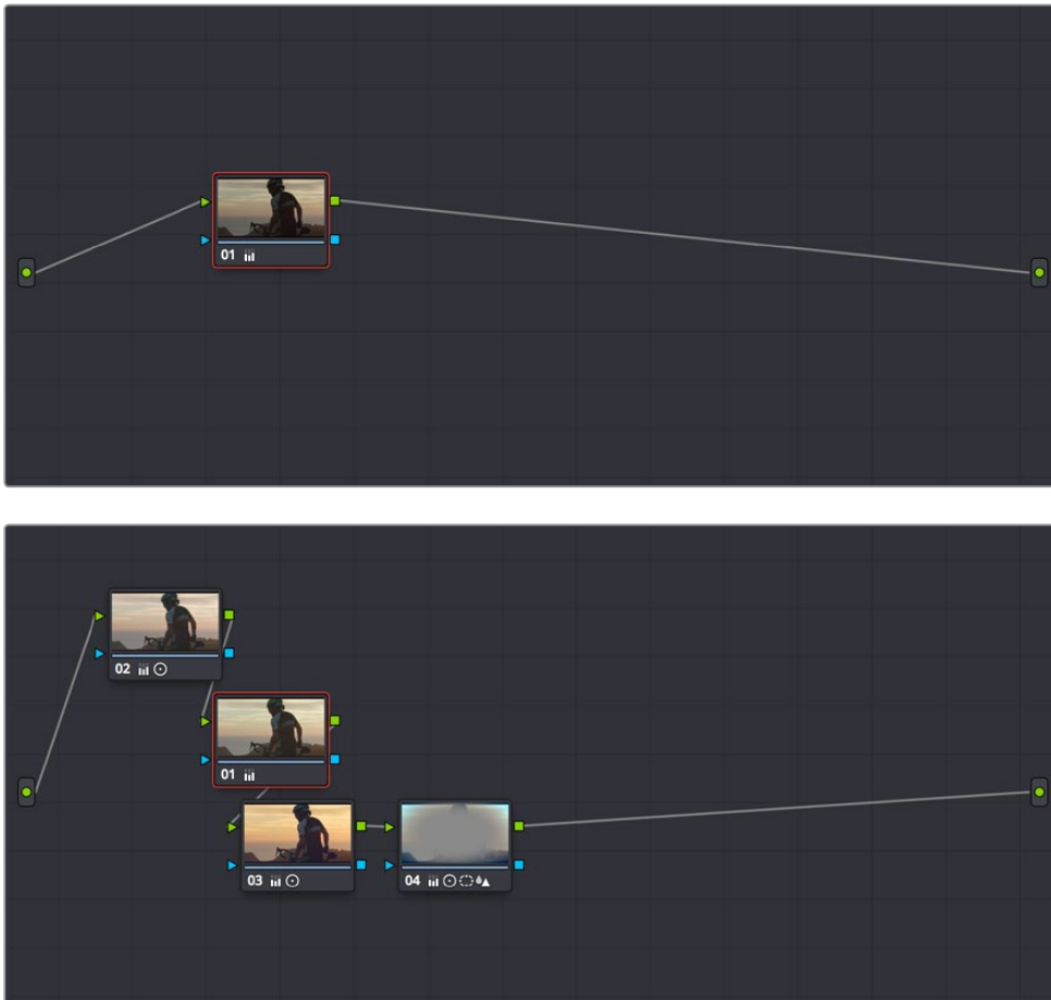
(Top) The Clip node tree, (Bottom) After using the Collapse Group Grades command to flatten the Pre-Group and Post-Group nodes into the Clip node tree
