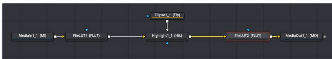
A node tree with “to linear” conversions at the beginning, and a “from linear” conversion at the end
