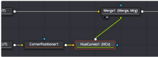
Adding the HueCurves node to make a correction to the foreground image
