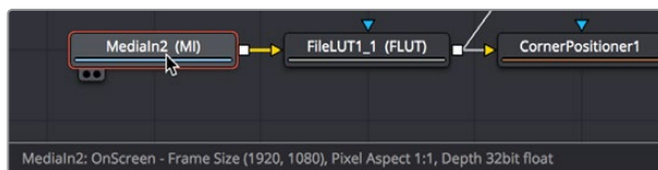
The Status bar under the Node Editor showing you information about a node under the pointer
