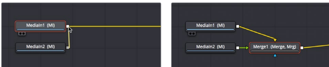
(Left) Dragging a connection from a disconnected node to another node's output, (Right) Dropping it to create a Merge node composite
