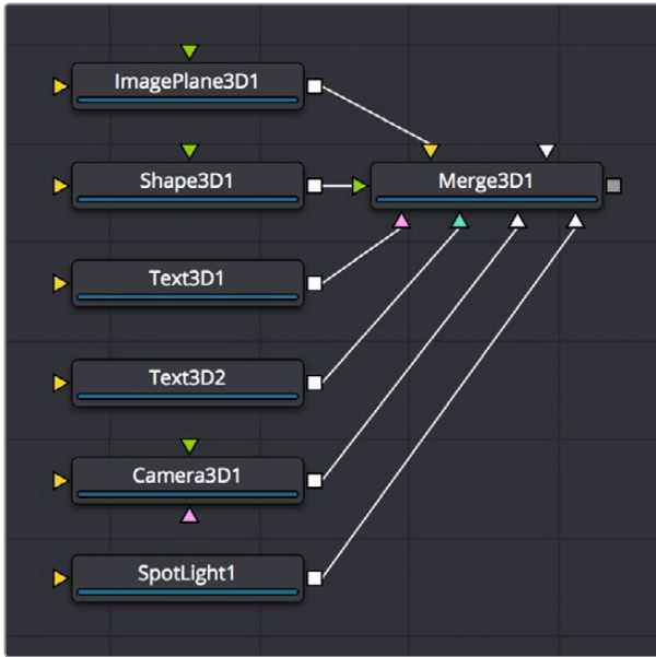
After dragging a connection line and dropping it on top of a Merge3D node
