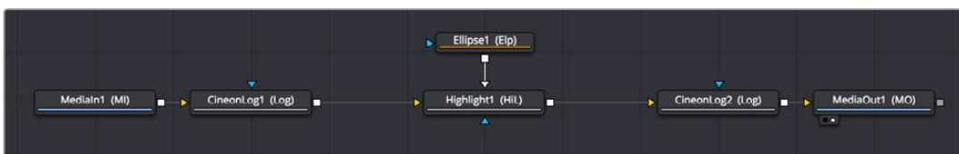
Converting all images to linear coming into the composite, and converting out of linear out of the composite, in this case using CineonLog nodes at the beginning and end
