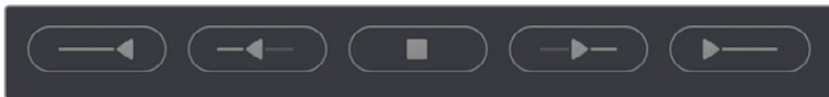
The analysis buttons, left to right, Track from Last Frame, Track Backward, Stop Tracking, Track Forward, Track from First Frame
