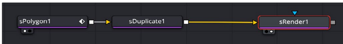
An sPolygon node connecting to an sDuplicate node, and then viewed using an sRender node
