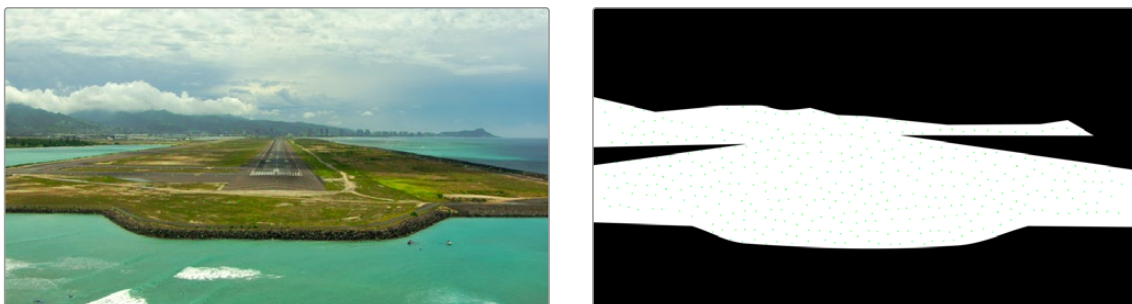
The original image to be tracked (left), and the occlusion mask of the clouds and water (right)
