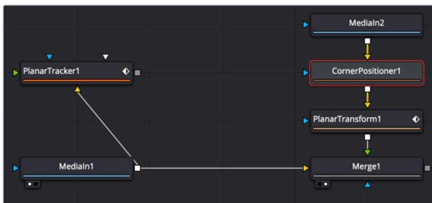
The Corner Positioner corner pins a clip in place and uses a Planar Transform to match move it to the background.
