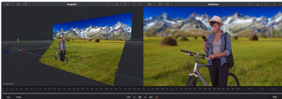
Side-by-side dual viewers: a 3D viewer (left), and a 2D viewer (right)
