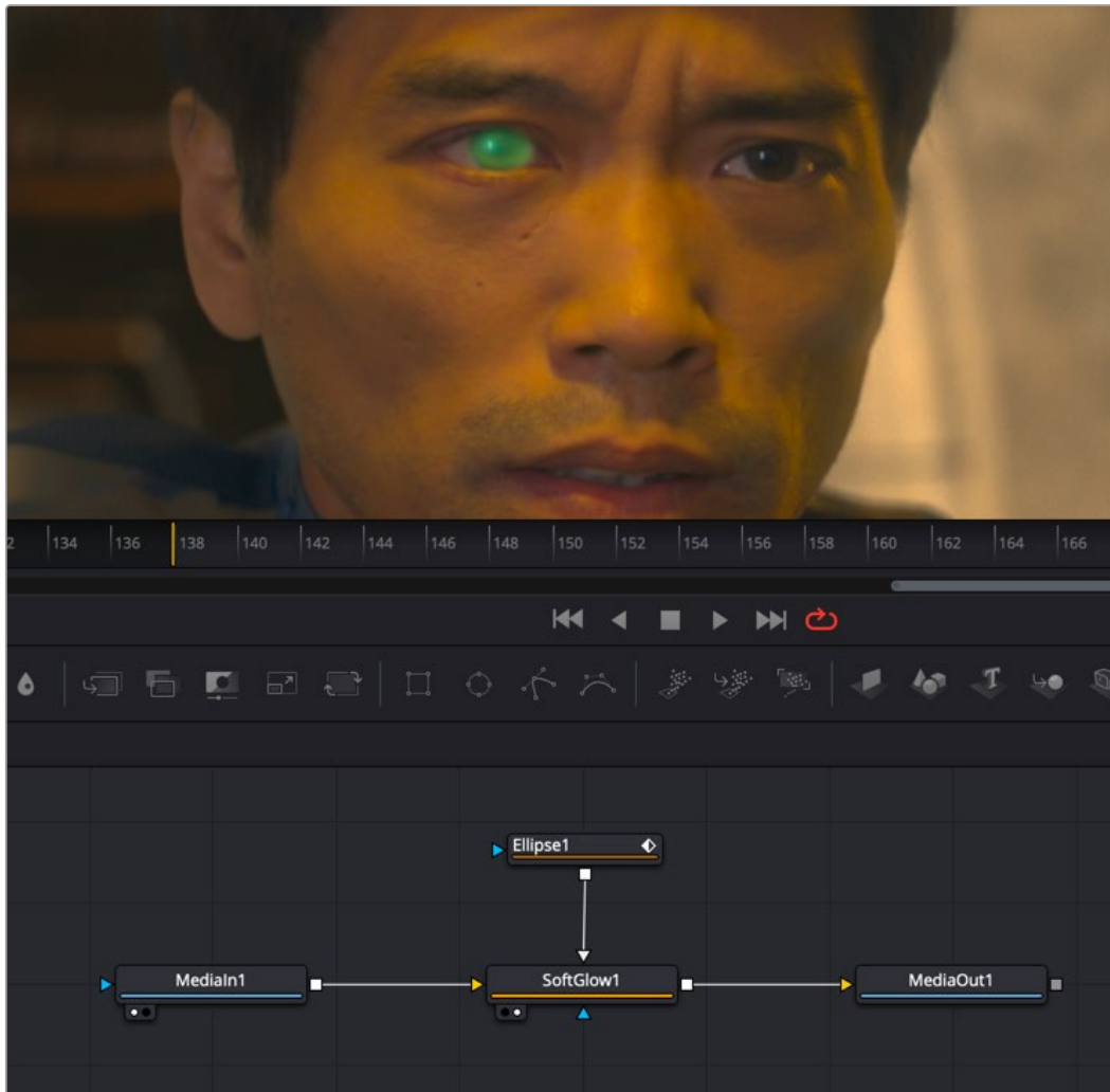
A Tracker modifier applied to the Ellipse to create a green glow on an actor's pupil
