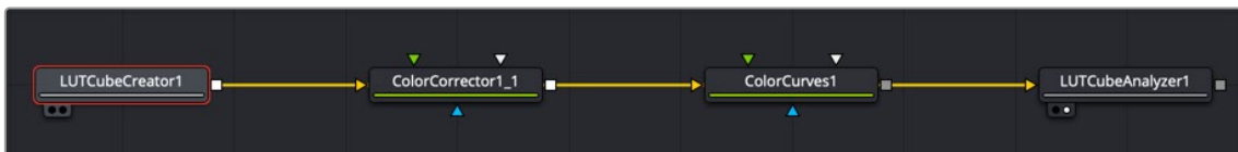
Generating a LUT starts with the LUT Cube Creator and ends with a LUT Cube Analyzer.
