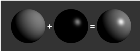
Three spheres, left to right: diffuse only, specular only, and combined
