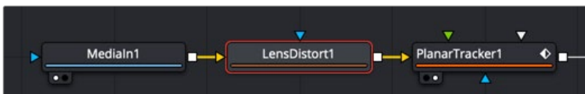
A Lens Distort node inserted between a MediaIn1 and Planar Tracker to remove lens distortion
