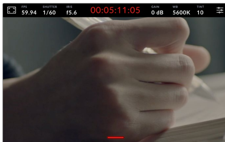
Swipe up or down to hide lower third overlays on the LCD touchscreen
