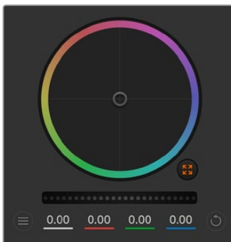
Adjust the master wheels by dragging the wheel control left or right
