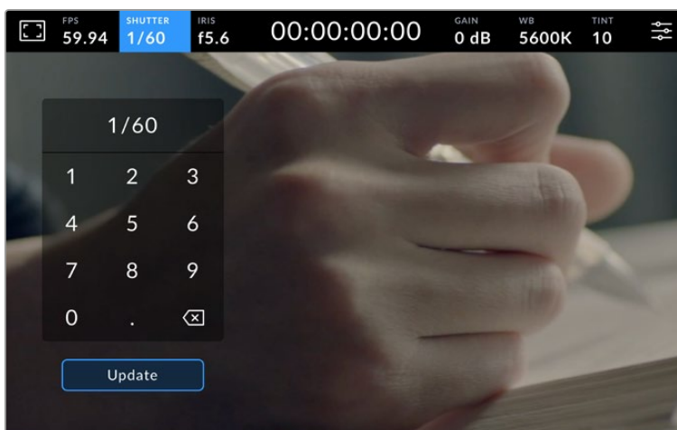
Use the manual shutter keypad to enter your shutter timing of choice when shooting outdoors or under flicker free lights
