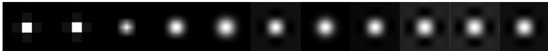
Resizeフィルター (左から) : Nearest Neighbor, Box, Linear, Quadratic, Cubic, Catmull-Rom, Gaussian, Mitchell, Lanczos, Sinc, Bessel
