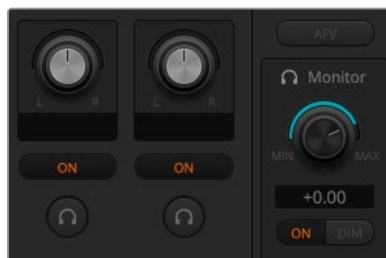
The monitor volume knob and buttons set independent audio levels and allow solo monitoring on the monitor XLR output
