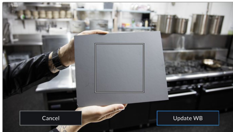
Tapping the 'AWB' icon in the white balance menu will bring up the auto white balance screen. Use this with a white or neutral gray surface to automatically set a neutral white balance
