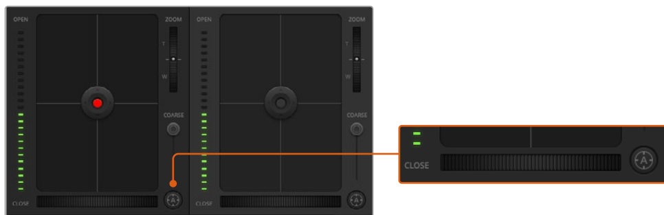
Click on the auto focus button or drag the manual focus adjustment left or right to focus a compatible lens
