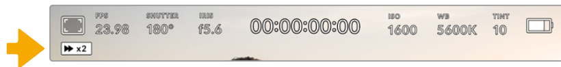
The shuttle speed indicator displays the speed and direction of footage being fast forwarded or reversed
