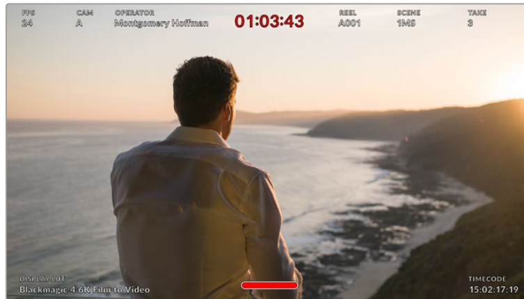
Your URSA Mini can display director specific status text on its front and main SDI outputs
