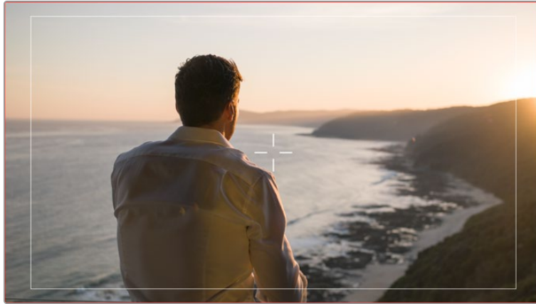
When connected to an ATEM switcher sending a tally signal, a red border will appear around your camera's image preview when grids are set to 'on'
