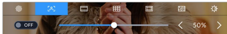
Tap the 'focus assist' icon while accessing 'LCD monitor options' to access your camera's focus assist settings
