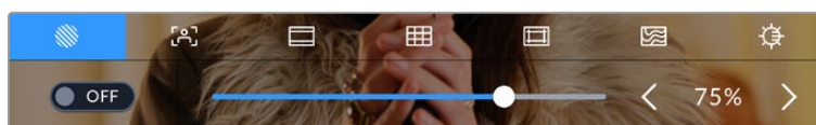
Tap the 'zebra' icon while accessing 'LCD monitor options' to access the zebra settings
