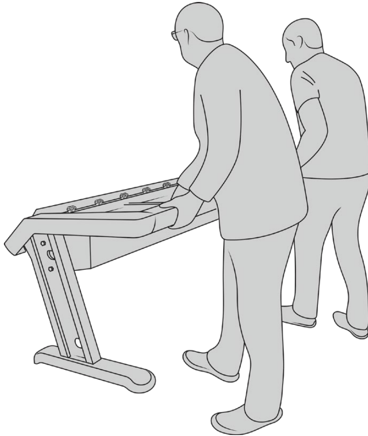
Lean the Fairlight console onto its feet, ready to install the Fairlight panels
