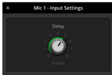
Click on the delay control and drag left or right to decrease or increase the amount of delay required for an analog input
