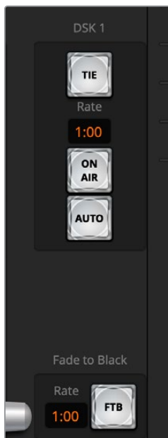
Downstream key and fade to black
