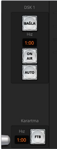
Downstream key ve karartma
