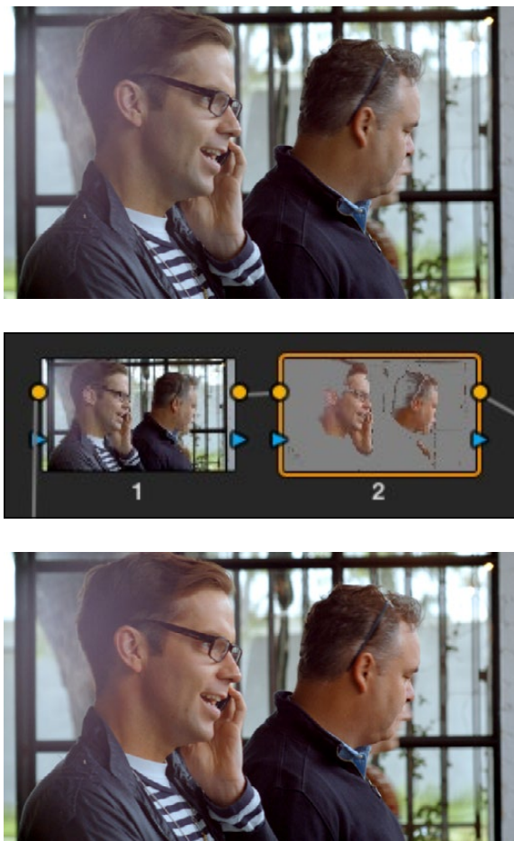
Top—The image with a simple primary correction. Middle—Adding a second node and using HSL Qualification to isolate the skin tones. Bottom—The final adjusted image.
