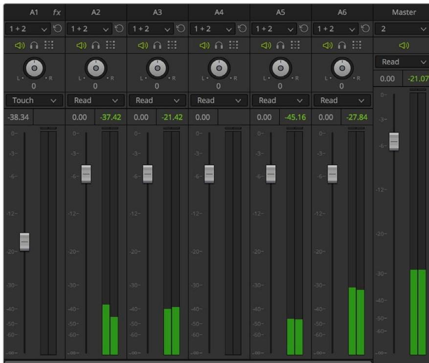
The Audio Mixer, with four channel strips corresponding to the four tracks in the Timeline
