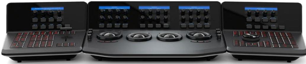
All three panels have LCD panels which display the menus
