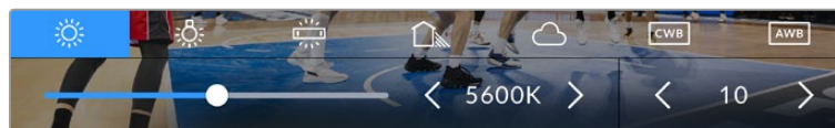
The white balance and tint indicator on your Micro Studio Camera 4K G2 gives you access to five presets
