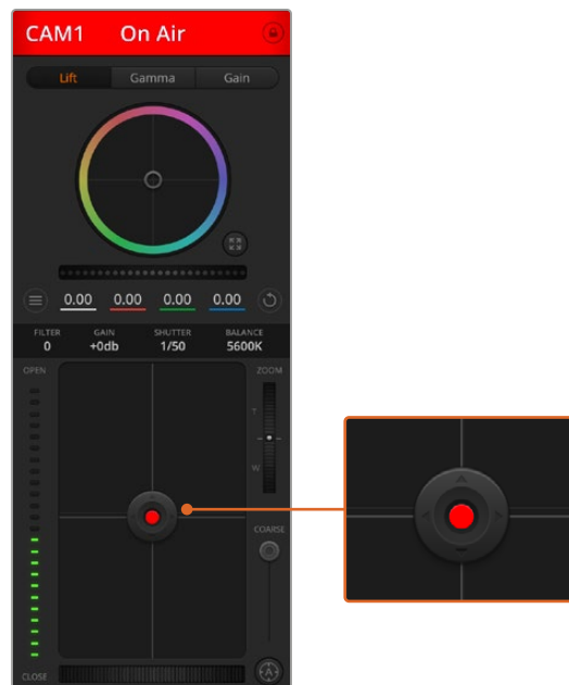
The iris/pedestal control illuminates red when its respective camera is on air
