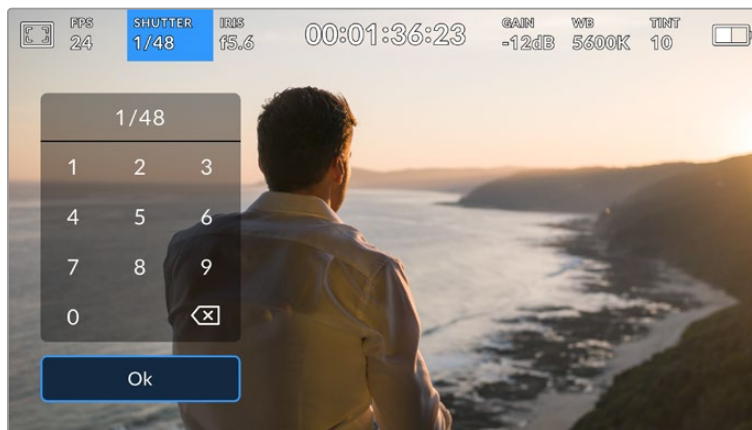
The manual shutter keypad allows you to type in any shutter value you wish
