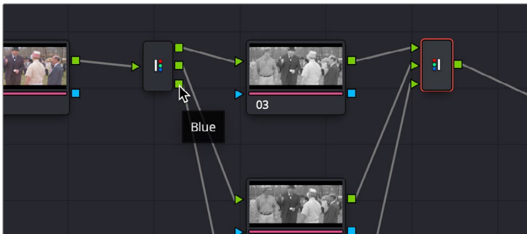
Hovering the pointer over a Splitter Node's output will tell you the color channel of that output.
