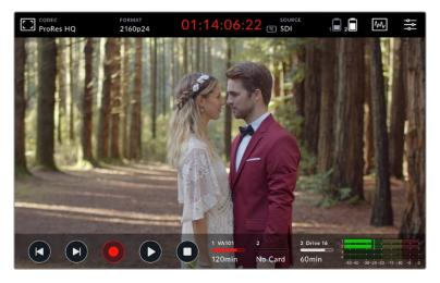
The timecode display in the upper toolbar will illuminate red while recording
