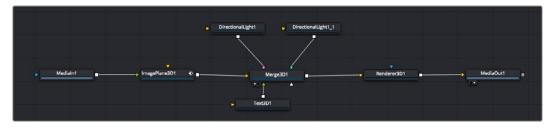
The most commonly used tool is the 2D or 3D merge node. This node is like a central hub that combines tools on the node editor into a single output.
