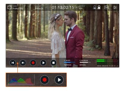
The lower toolbar includes transport controls, storage indicators and audio meters. A display histogram can also be turned on via the menu to appear over the skip buttons on the lower left of the toolbar.
