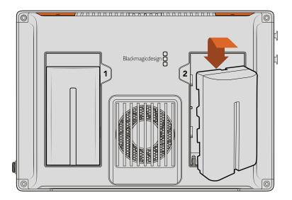
Insert the battery into the slot and slide down until it clicks into place. To remove, press and hold the button above the battery and slide the battery out
