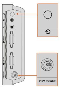
Connect external power to the +12V power input. Press the power button to turn the unit on.
