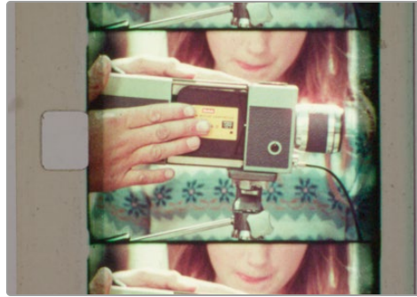
Incorrect setup shows the aperture shutters are set too narrow resulting in dark areas on both sides of the image
