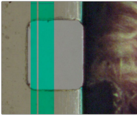
Incorrect 8mm setup. The overlay is not aligned to the edge of the perforation.
