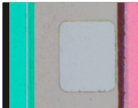
Correct 8mm setup. For the stabilization overlay, the transparent stripe in the overlay is within the film base area.
