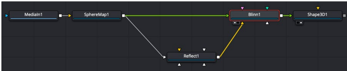
A Blinn shader with diffuse and specular color materials connected
