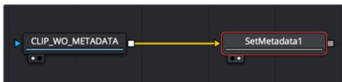
A Set Metadata node creates new metadata and embeds it into the background clip.
