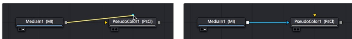
Side by side, dropping a connection on a specific node input, note how the inputs rearrange themselves afterwards to keep the node tree tidy-looking
