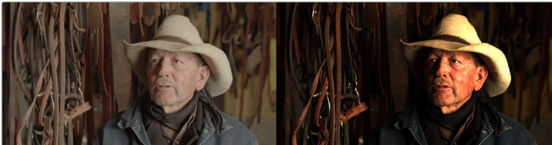
A clip displayed with a nonlinear, log gamma curve (left) and the clip transformed to linear gamma (right)
