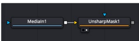
An Unsharp mask node applied to a MediaIn1 node
