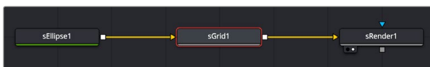
An sEllipse shape connected to an sGrid and then output to an sRender for viewing and combining with other elements
