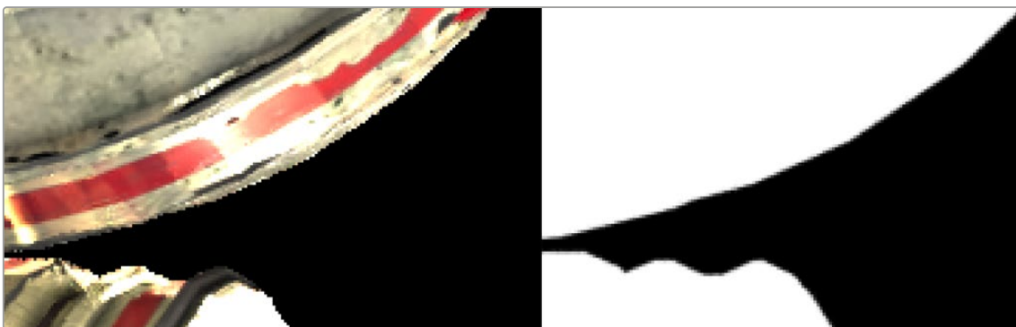
A detailed view of a non-premultiplied RGB image (left) and its alpha channel (right)
