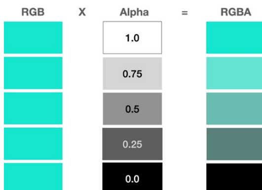
RGB pixels are multiplied by varying degrees of transparency and the result is a different RGB value.
