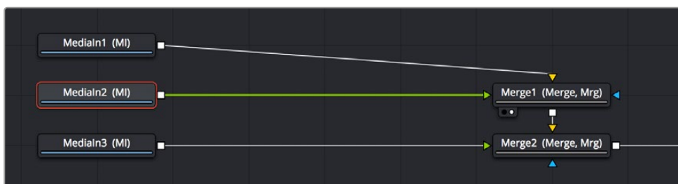
Creating space after the MediaIn nodes and selecting the second one in preparation for adding a node
