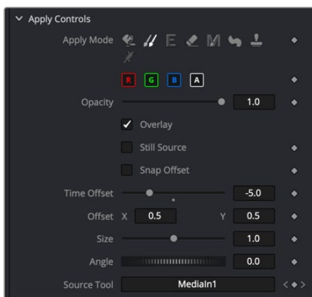
The Clone Apply Mode can use a different frame from the same clip
