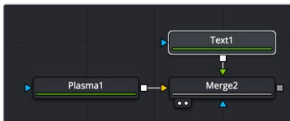
Text+ node connected as the foreground to a Merge node
