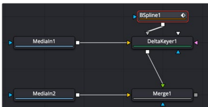
A B-Spline node generates a smooth, curved shape as a garbage matte
