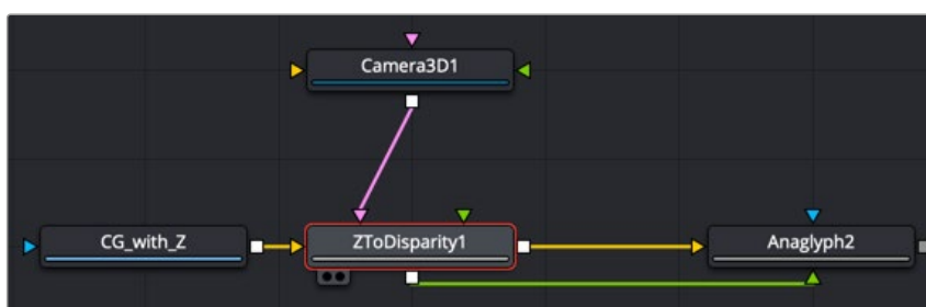
A Z To Disparity node takes an image with a Z channel and creates a disparity channel
