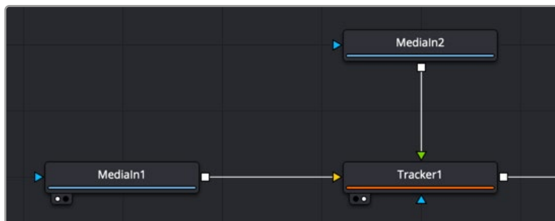
Connecting a MediaIn node's output to a Tracker node's background input
