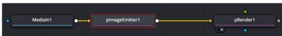
A plmage Emitter node emits particles based on an image connected to the orange input.
