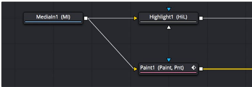
The Medialn node's output is branched but carries the same RGB channels to both inputs.
