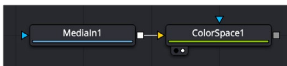
A Color Space node applies a conversion to a Medialn1 node
