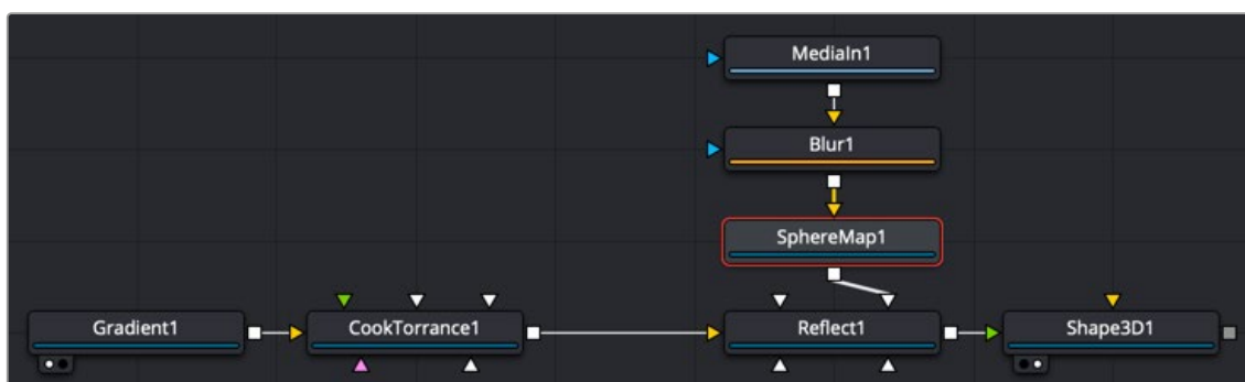
A Sphere Map node generates a reflective environment when connected to a Reflect node Reflection Color input.
