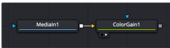
A Color Gain node applied to a Medialn1 node
