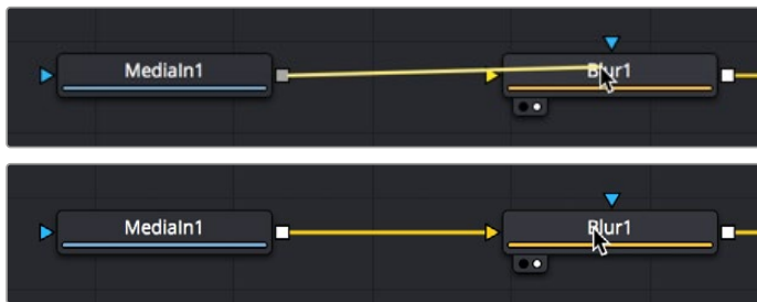
Before (top), and after (bottom) dragging a connection line and dropping it on top of a node.
