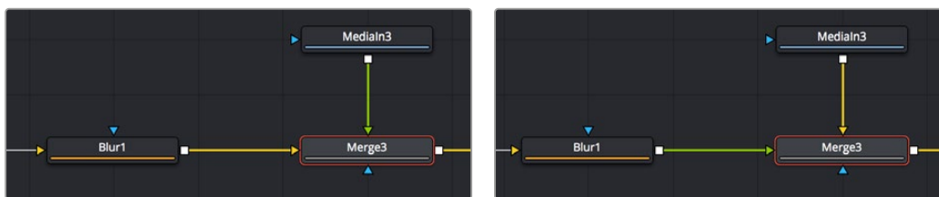
Before swapping node inputs (left), and after swapping node inputs (right), the connections don't move but the colors change.
