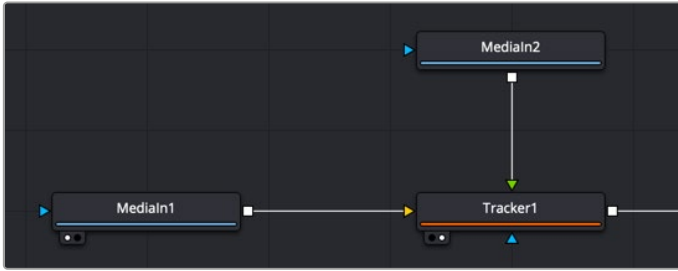
Tracker node connected serially so it can both track and transform the input images
