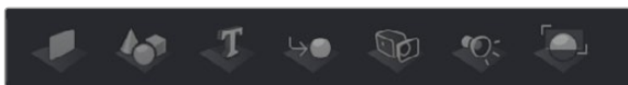
The 3D nodes available from the toolbar include the ImagePlane3D, Shape3D, Text3D, Merge3D, Camera3D, SpotLight3D, and Renderer3D nodes
