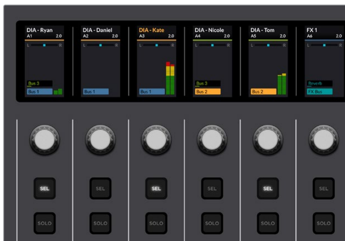
Strip mode Select buttons latched on tracks A1, A3, and A5, and the red track name on the A3 track indicating it is the active track
