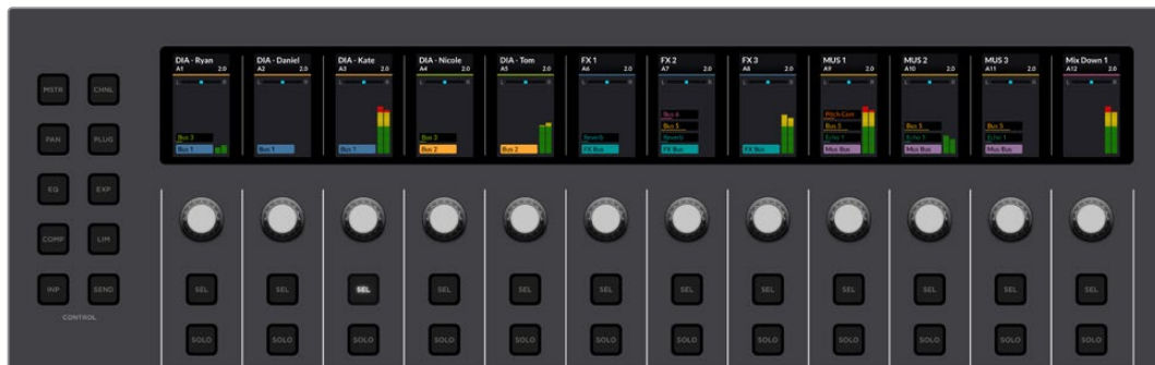
Default mode where SEL is Select button, knob controls Pan, and LCD shows channel info for each of the 12 channel strips.
