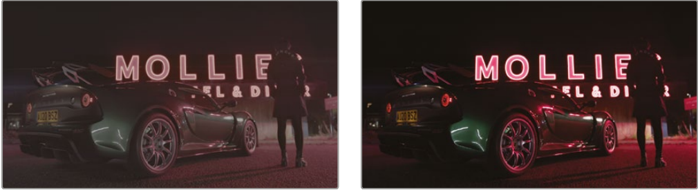
Log-encoded source (left) and the same source color managed to a deliverable color profile (right).
