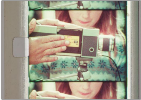
Incorrect setup shows the aperture shutters are set too wide resulting in light areas on both sides of the image
