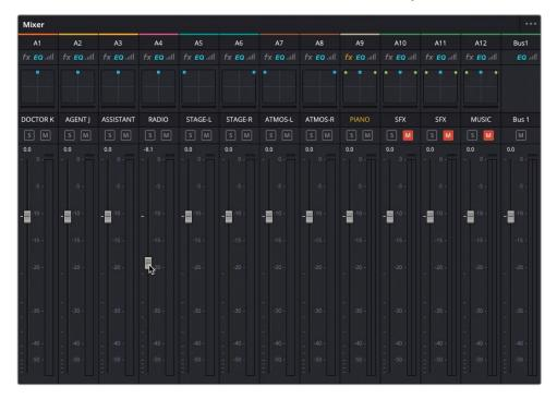
**TIP** You can see the relative adjustments you're making to the track's levels at the top of the slider controls.
