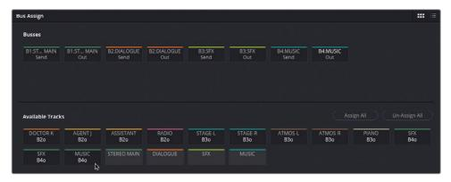
**TIP** To remove a track from a specific bus, click the bus from the Available Tracks section of the Bus Assign window, and then click the track. Tracks already assigned to the selected bus will be removed.
