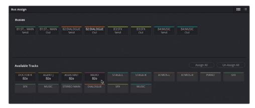
B2o (Bus 2 out) appears below the name of each track to identify which bus it is being routed to.
