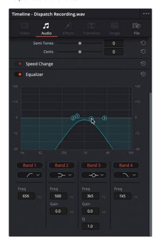
These changes limit the range of frequencies in the voice to just the midrange, making the clip sound a little tinny and artificial.
