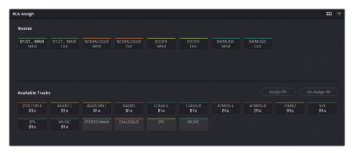
The Bus Assign window is used to view and change the destination of the audio once it leaves a track. By default, all audio tracks are automatically routed directly to Bus 1, abbreviated as B1o (Bus 1 out). This is ultimately what you are listening to when the timeline plays.
